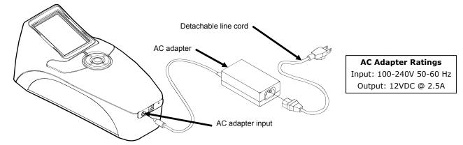
Operational hazard exists if an AC adapter other than X-Rite SE30-177L is used. Use only X-Rite battery pack SE15-38; other types may burst causing personal injury.
