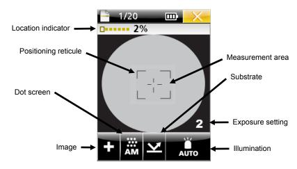
6. Locate the instrument's target window on the **2% patch** of the target strip using the reticule icon in the screen for positioning.
