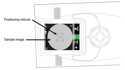
The instrument must be positioned flat on the sample and remain still through the entire measurement.
