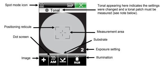
3. Position the instrument's target window on the sample using the reticule icon in the display for positioning. Make sure the sample is flat and the instrument is making good contact.
